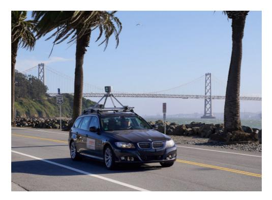
The Dutch company rigged a fleet of cars with cameras, radars, and light detection and ranging (LIDAR) units, the same stuff actual self-driving cars will have. As a carbon-based lifeform drives, the sensors collect data with such accuracy that a car using it will determine its position to within an inch.
